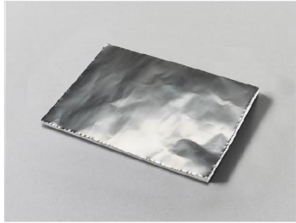
Fig.: Silica fleece (up to 1,000°C) Source Steinbach AG
